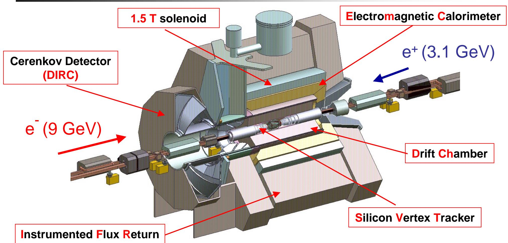
SVT: 97% efficiency,  $15 \mu\text{m}$  z hit resolution (inner layers, perp. tracks)
