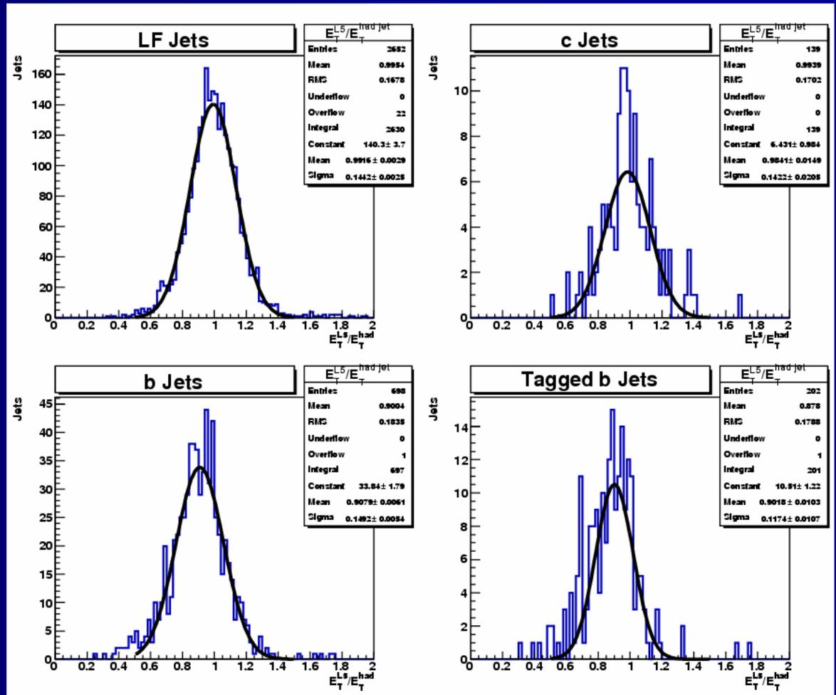
Measured  $b$ -jet energies are  $\sim 10\%$  low on average wrt “truth”.
