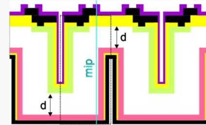
**IRST/CNM** fabricated in the RD50 Framework in 2005 Tested with SCTA readout Electronics. Data and Simulations show that the design is **NOT radiation hard** For B-layer replacement.
