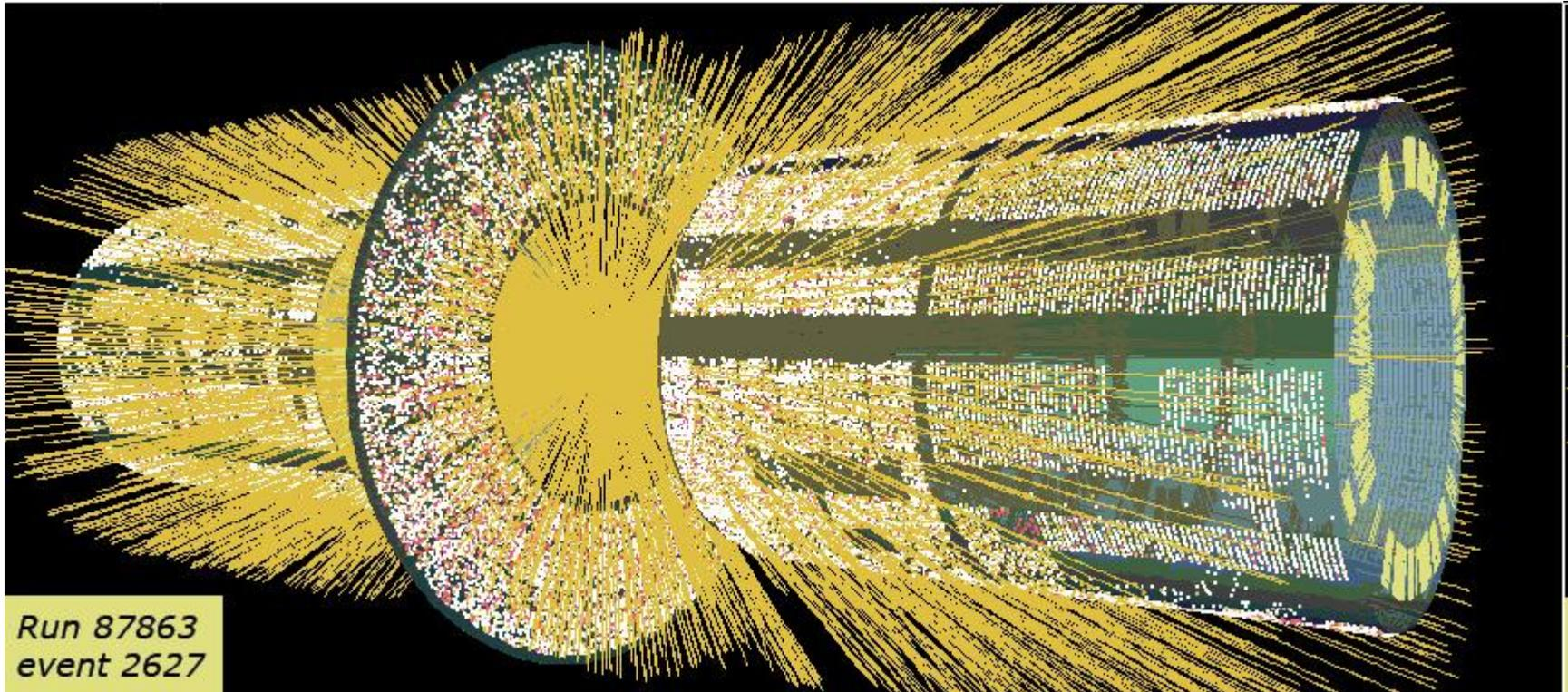
September 10, 2008 - A 'splash event' as ATLAS detects particles from nearby collisions from the first beams through the LHC
