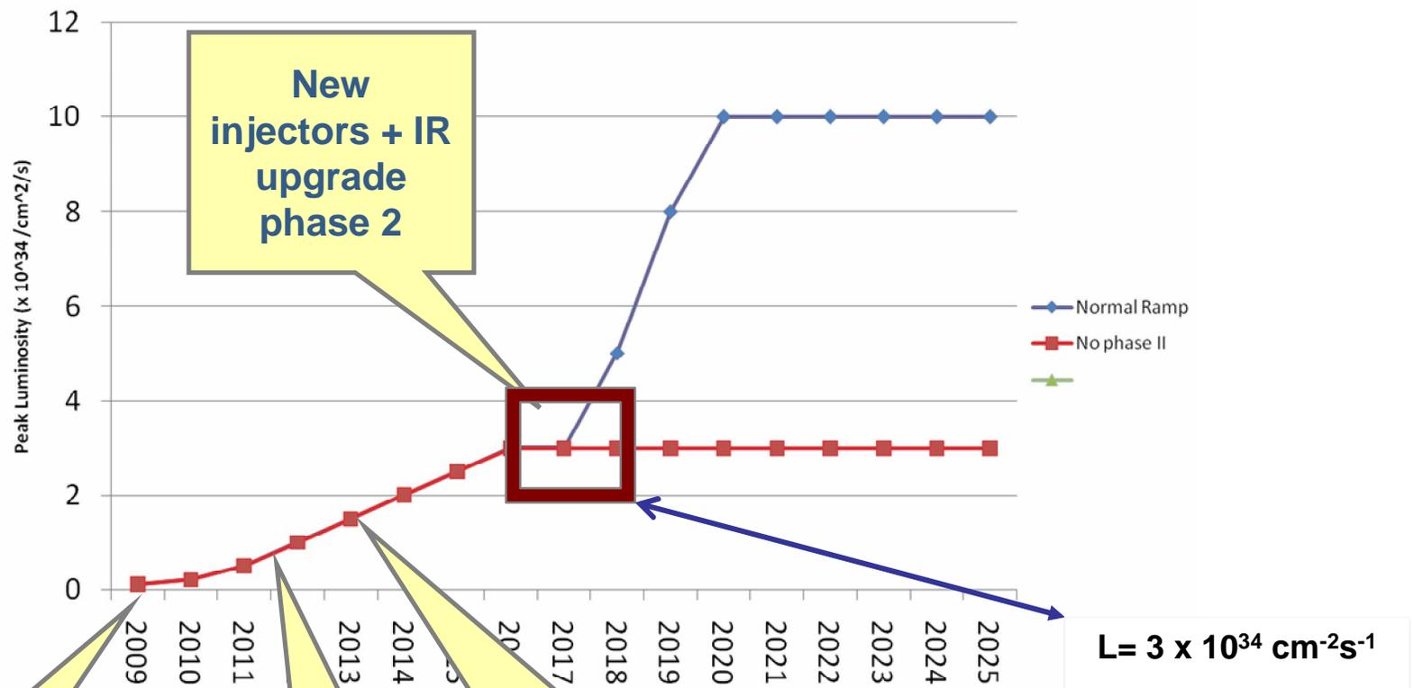
Detector robustness and performance have to fight for an higher than the today BL design luminosity ( $2 \times 10^{34}$ ) at a smaller radius (3.7 cm instead 5.0 cm)
