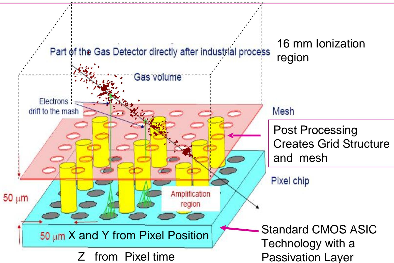
Ingrid is essentially a High Rate mini - Time Projection Chamber
