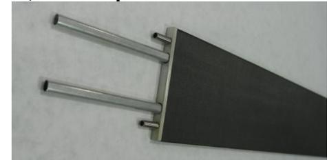
1.2 meter, 2.5 cm strip, 48 segments/side ~250-300 Watts (@0.25 W/chip)
