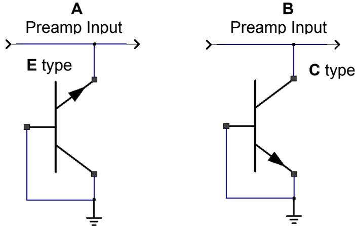
**Figure 1** Two configurations of the DMILL NPN transistor used for input protection of the ASDBLR. The large input transistors in the Common Emitter preamp assure that the input will not rise much above  $800\text{mV}$  so the potential difficulty of exceeding the maximum  $V_{be}$  reverse specification of a few volts is not a problem for configuration A.
