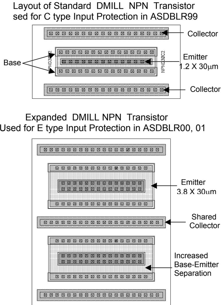
**Figure 3** The layout of a stretched DMILL transistor used for input protection in the ASDBLR99 is shown at the top of the figure. In ASDBLR99 the collectors were connected to the input (C type protection). The lower part of the figure shows a revised NPN layout implemented in ASDBLR00 for E type protection. In ASDBLR01 these (lower object) transistors were rewired and configured differently on different channels. Both E and C type protection have been implemented.
