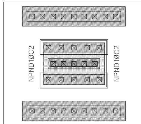
**Figure 2** Layout of Standard DMILL NPN transistor. Emitter stripe contact, center, base contact stripes on either side of emitter and collector contacts are the outer two stripes.
