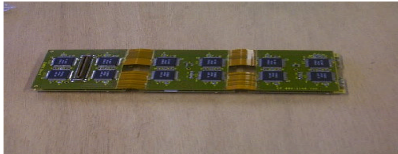
Figure 3: Flex-rigid front-end board with 12 DTMROC and 24 ASDBLR chips (192 channels).
