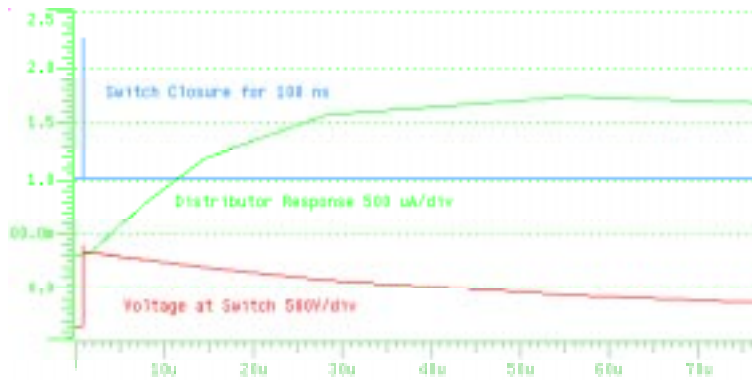
FIGURE 9. 100ns Switch Time, 200m cable, 10k x 10nF filter
