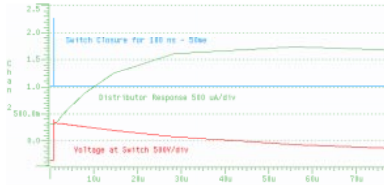
FIGURE 12. Change Cable from 200m to 50m
