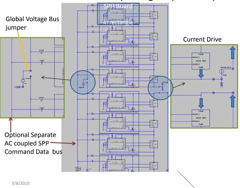
Schematically wired SPP and ABCn for two Loops
