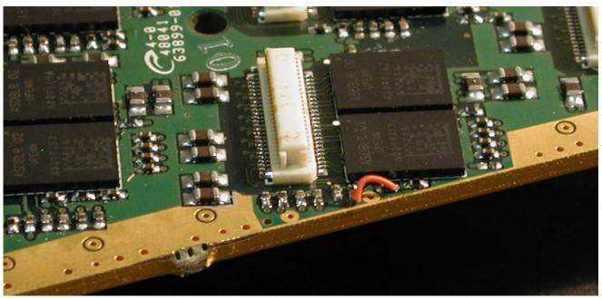
Closeup view of installed jumper. Note jumper attaches to 4.7ohm resistor on contact away from the ASDBLR chip, towards perimeter of board.
