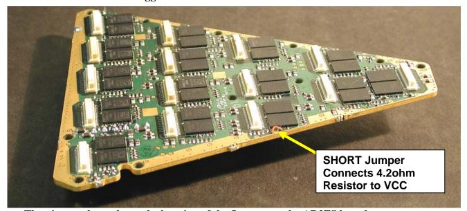
The picture above shows the location of the Jumper on the AR2FS board.
